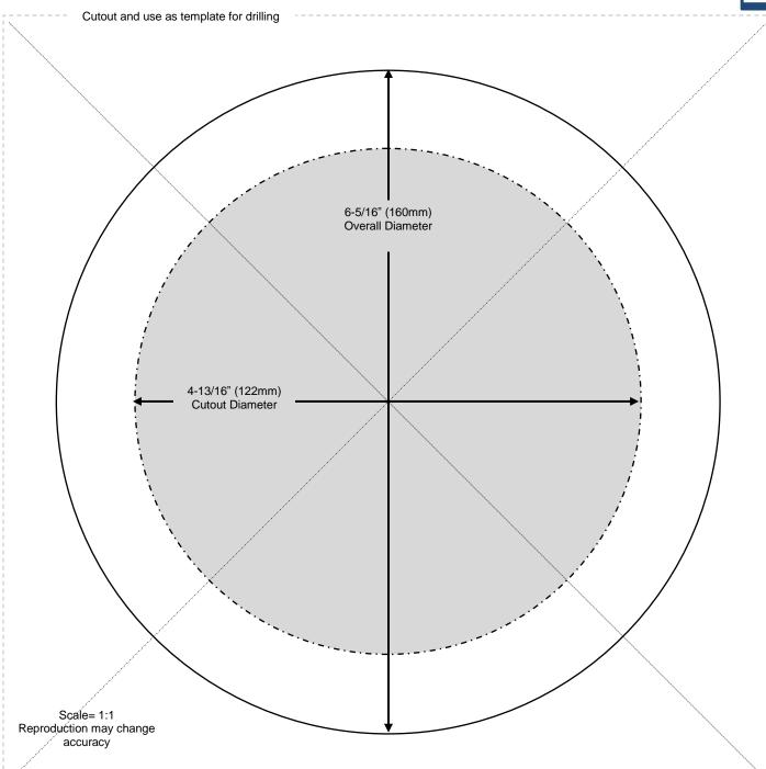
**Installation:** Find a suitable location making sure there is clearance for the installed depth. Use a hole saw or other suitable device to make a cutout.
